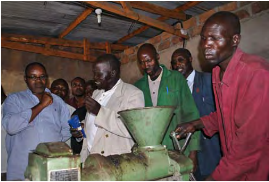
Mr. Livingstone Otwane, Chairman of the CPC in Changara, explains to the UNDP Resident Representative, Aeneas Chuma the process of extracting sunflower oil for the bio-diesel generator at the centre ©UNDP 2011
